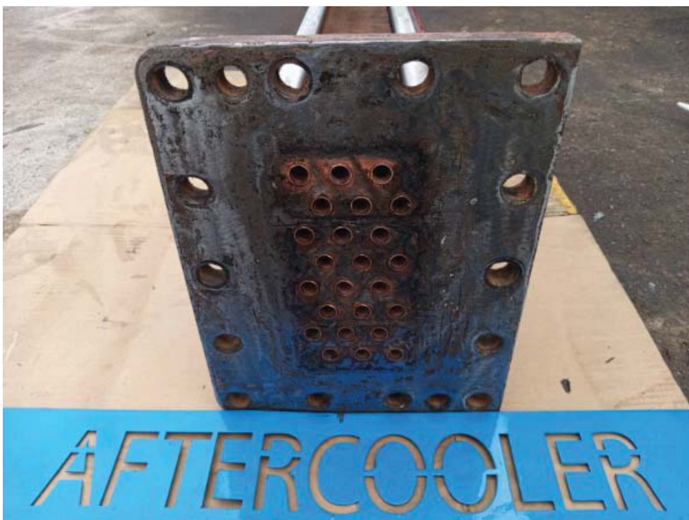
AFTERCOOLER AFTER CLEANING
