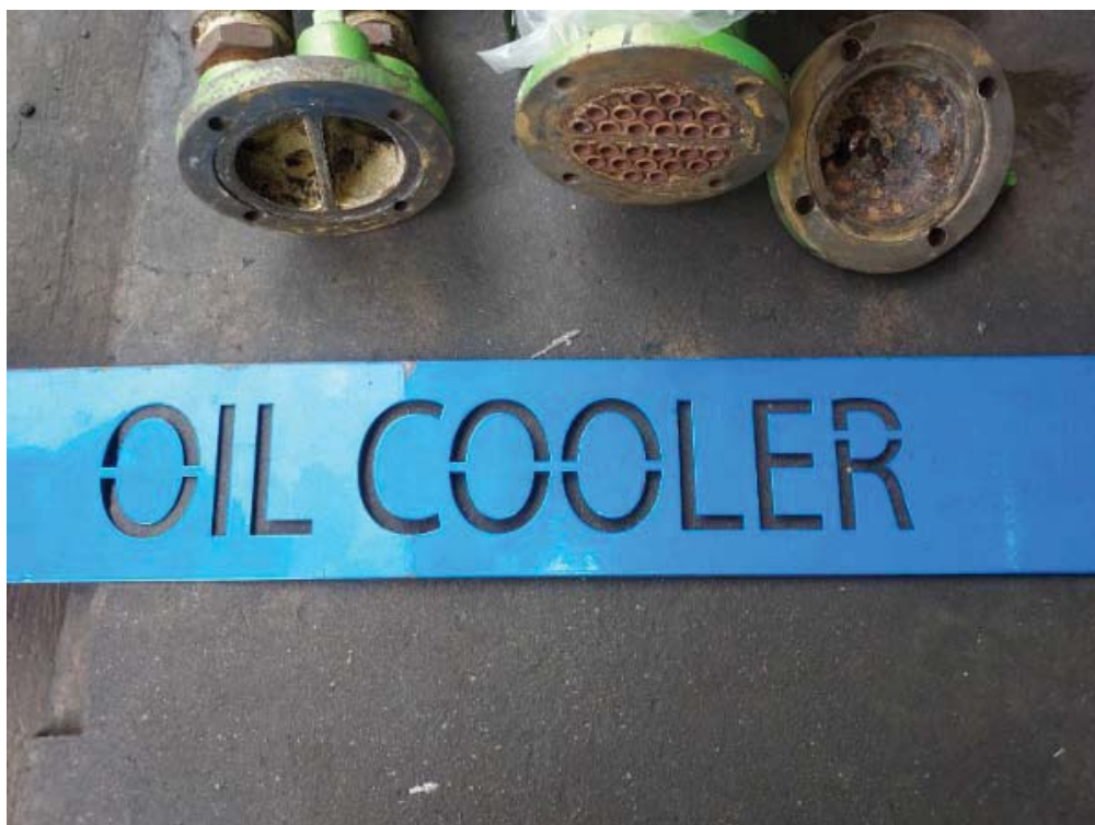
OIL COOLER AFTER CLEANING
