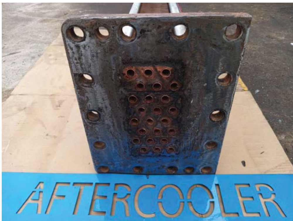
AFTERCOOLER AFTER CLEANING
