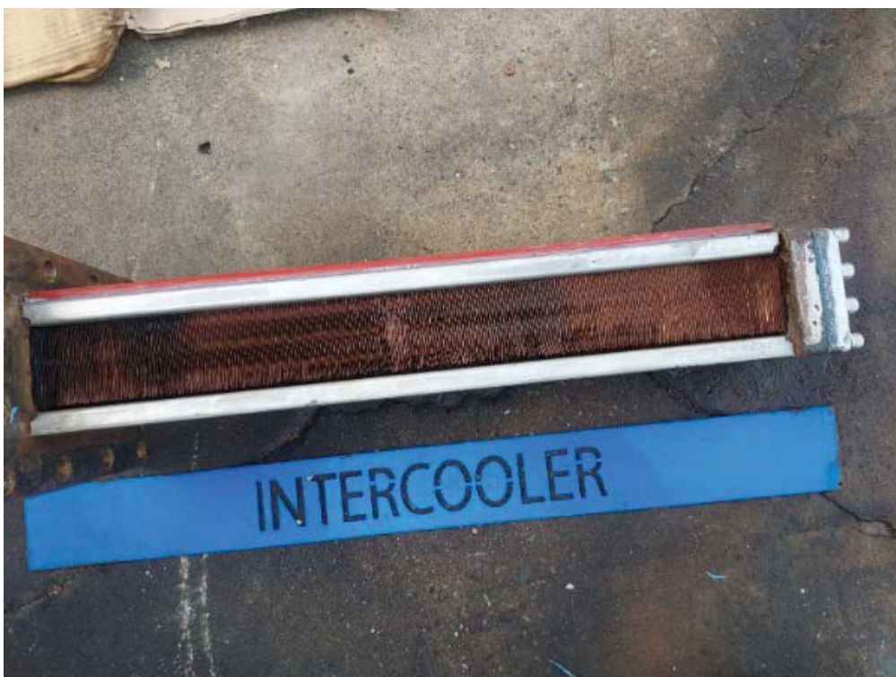
INTERCOOLER AFTER CLEANING
