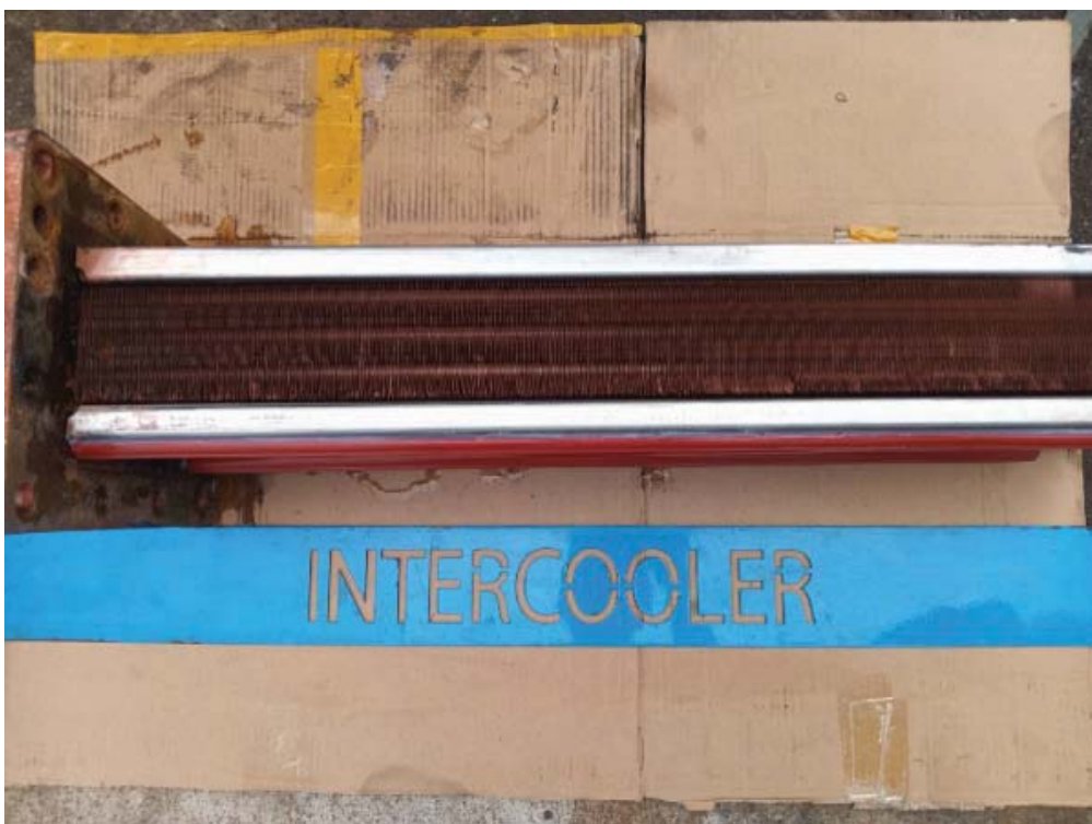
INTERCOOLER AFTER CLEANING
