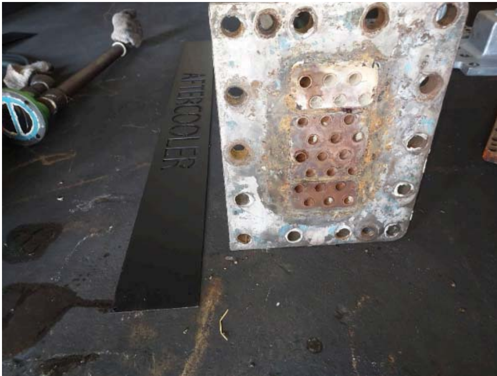
AFTERCOOLER BEFORE CLEANING
