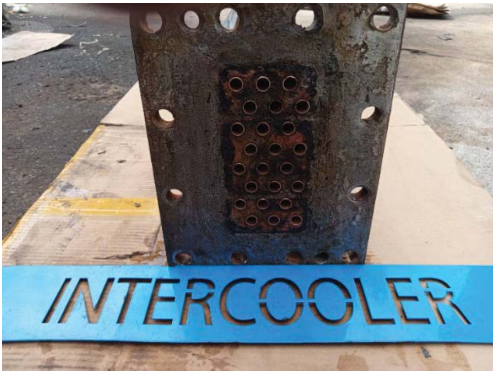
INTERCOOLER AFTER CLEANING
