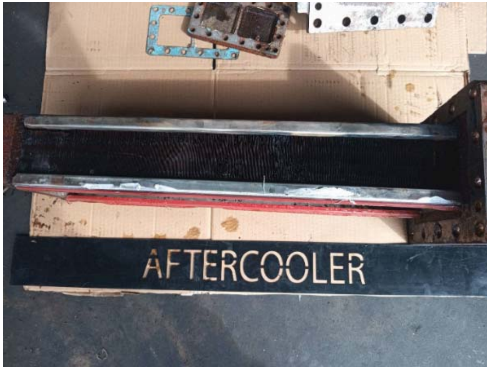
AFTERCOOLER BEFORE CLEANING
