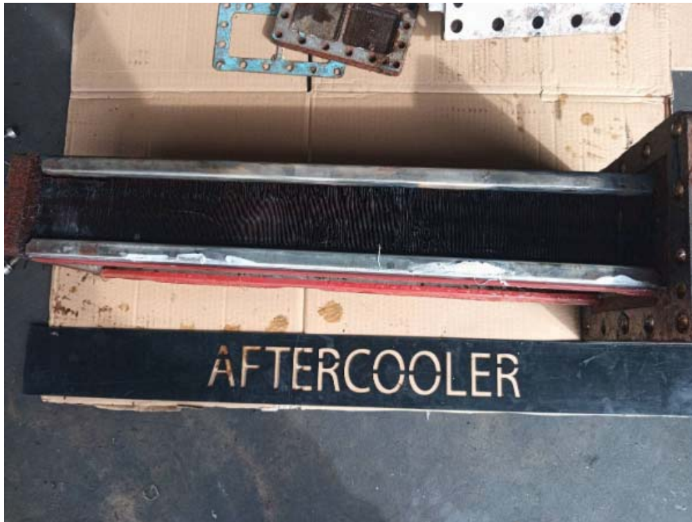
AFTERCOOLER BEFORE CLEANING
