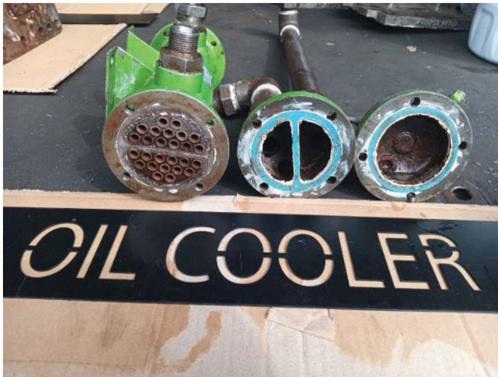
OIL COOLER BEFORE CLEANING
