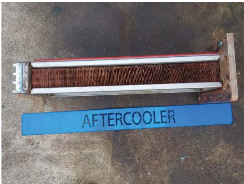
AFTERCOOLER AFTER CLEANING
